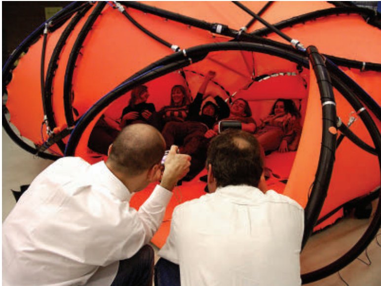
► Figure 4. MuscleBody is a continuous tensile textile stretched inside a tubing structure that is driven by pneumatic “muscles” that change its shape and thereby skin transparency. Credit: Hyperbody, Faculty of Architecture, TU Delft, 2005
