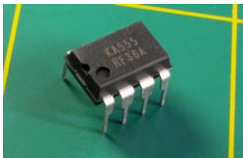
Figure 4-2. An integrated circuit chip in Plastic Dual-Inline Pin package, abbreviated PDIP, or, more often, DIP.
