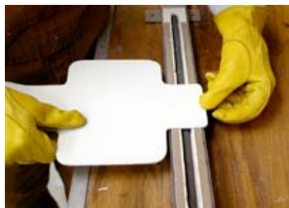
Figure 5-85. Making clean, precise bends in ABS is simply a matter of resting the plastic over a bender that consists of an electric heating element.
