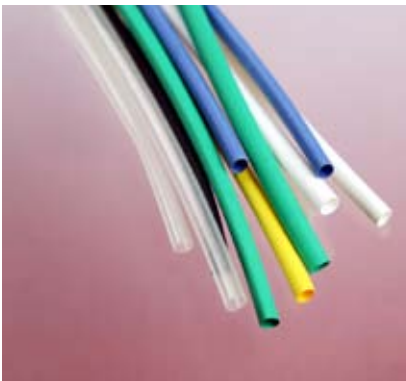
Figure 3-21. Slide heat-shrink tubing over a bare joint and apply heat from a heat gun to make a tight insulating seal around the joint.
