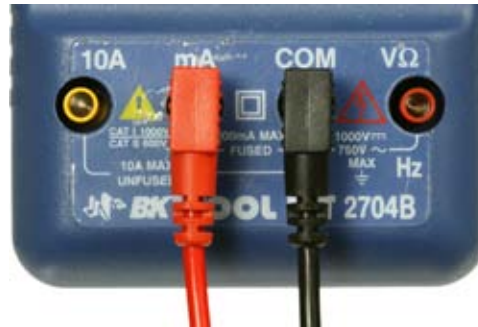
Figure 1-61. A manual meter such as the one here may require you to shift the red lead to a different socket, to measure milliamps. Most modern meters don’t require this until you are measuring higher currents.
