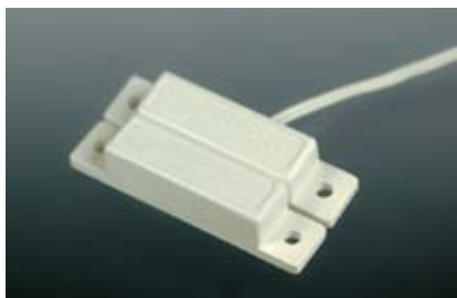
Figure 3-85. In this simple alarm sensor switch, the lower module contains a magnet, which opens and closes a reed switch sealed into the upper module.
