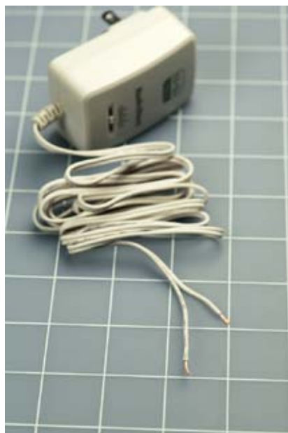
Figure 2-50. Second, strip the wires, making one shorter than the other to reduce the risk of them touching. Color one of the adapter wires red with a marker, to identify it as the positive one.
