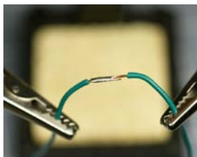
Figure 3-44. The finished joint has enough solder for strength, but not so much solder that it will prevent heat-shrink tubing from sliding over it.
