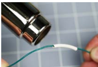
Figure 3-49. Apply heat to the tubing.
