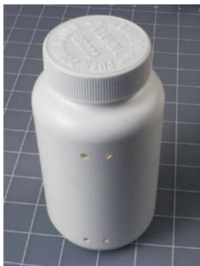
Figure 5-60. A large, 3-inch diameter empty vitamin bottle makes an ideal core for a crystal radio coil. The drilled holes will anchor wire wrapped around the bottle.
