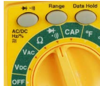
Figure 2-32. To check a circuit for continuity, turn the dial of your meter to the symbol shown. Only use this feature when there is no power in the component or the circuit that you are testing.
