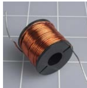
Figure 5-46. The black tape is removed, revealing a coil of magnet wire.
