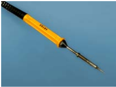
Figure 3-1. The low wattage of this pencil-style soldering iron enables you to use it safely on sensitive components, and the sharp tip helps to apply heat selectively.
