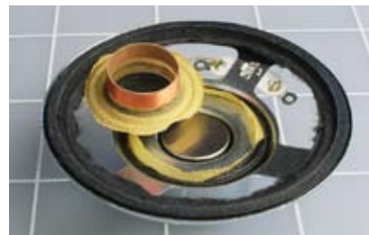
Figure 5-27. The neck of the cone has been pulled out. Note the coil of copper wire, which fits precisely in the groove between two magnets in the base of the speaker.
