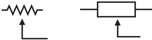
Figure 2-42. Potentiometer symbols: the left is traditional and used in the United States, the right is European. In both cases the arrow indicates the wiper (usually the center terminal).
