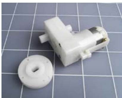
Figure 5-75. For the Little Robot Cart, I found this 5-volt motor, which is supplied with a disc that fits its output shaft. The combination cost less than $10.
