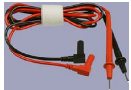
Figure 1-17. The black lead plugs into the Common (COM) socket, and the red lead plugs into the red socket that's almost always on the righthand side of a multimeter.
