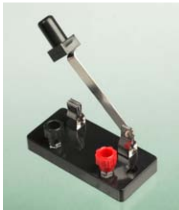
Figure 2-25. A single-pole, single-throw switch makes only one connection with one pole. Its two states are simply open and closed, on and off.
