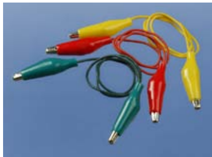
Figure 2-10. Patch cords, sometimes known as test leads, consist of wires preattached to alligator clips. This is another of those little luxuries that reduces the hassle factor in hobby electronics.
