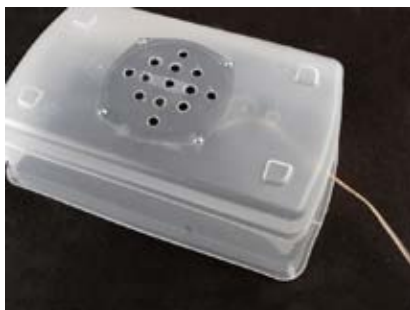
Figure 5-40. Drill some half-inch holes in the bottom of the box, then bolt the speaker in place, running a wire out through a hole in one end. Snap on the lid, and you're ready for not-quite-high-fidelity audio.
