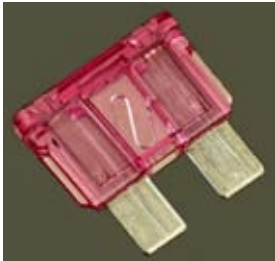
Figure 1-12. A 3-amp fuse intended primarily for automotive use, shown here larger than actual size.
