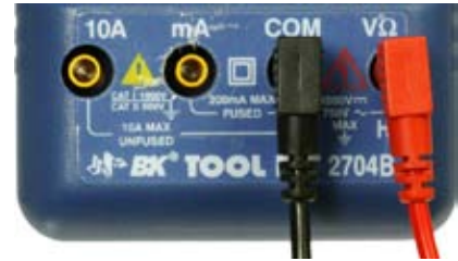
Figure 1-20. To measure resistance and voltage, plug the black lead into the Common socket and the red lead into the Volts socket. Almost all meters have a separate socket where you must plug the red lead when you measure large currents in amps, but we’ll be dealing with this later.
