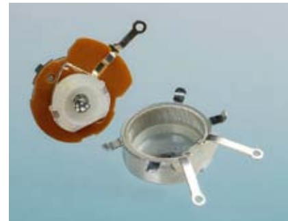
Figure 1-48. To open the potentiometer, first pry up the four little metal tabs around the edge (you can see one sticking out at the left and another one sticking out at the right in Figure 1-47). Inside is a coil of wire around a flat plastic band, and a pair of springy contacts (the wiper), which conduct electricity to or from any point in the coil when you turn the shaft.
