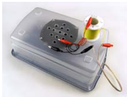
Figure 5-43. The red and black alligator clips, lying on top of the shoebox, should connect with the output from your amplifier chip. The red jumper wire passes the signal through a coil of hookup wire on its way to the speaker. Note the change in sound when you short out the coil.
