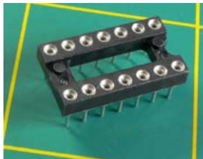
Figure 4-5. When you're soldering a circuit onto perforated board, sockets eliminate the risk of overheating integrated circuit chips and reduce the risk of zapping them with static electricity, and enable easy replacement.
