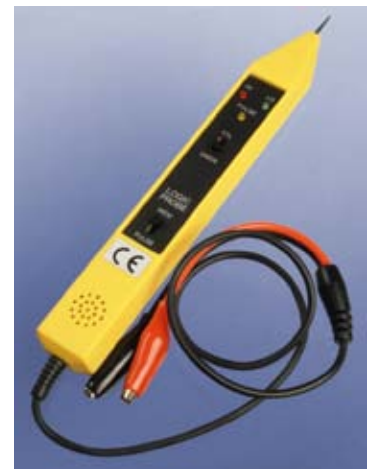
Figure 4-1. A logic probe detects the high or low voltage on each pin of a chip, and reveals pulses that may occur too quickly for you to perceive them with the unaided eye.
