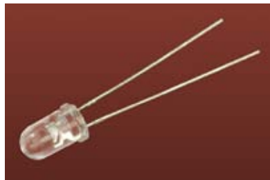
Figure 1-14. Typical 5-mm diameter light-emitting diode (LED).
