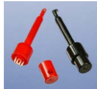
Figure 3-8. Then screw a collar over the protruding piece of wire, and screw on the cap. The other end of the wire is soldered to a probe.
