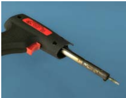
Figure 3-2. This higher-wattage soldering iron delivers the additional heat necessary for thicker wire or larger components. The discoloration quickly occurs as a result of everyday use and has no effect on the capability of the iron, as long as the tip of it is clean.
