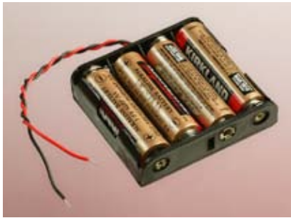
Figure 1-10. Battery carrier for four AA cells, to be installed in series, delivering 6 volts.
