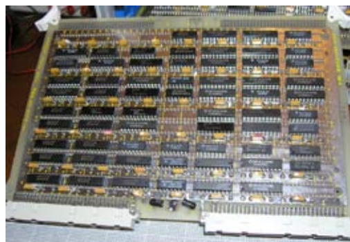
Figure 4-65. Hobbyist Bill Buzbee built himself a web server entirely from 7400 series logic chips, the oldest of which was fabricated back in 1969. The web server can be found online at http://magic-1.org , displaying pictures of itself and details of its construction. The picture here that Bill took shows just one of the circuit boards of this remarkable project.
