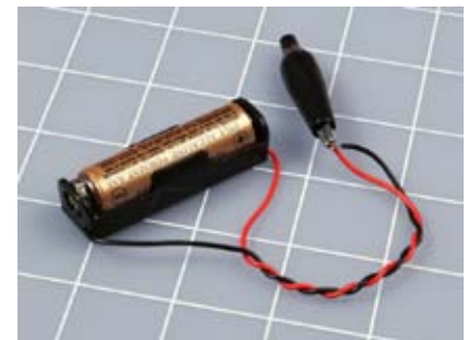
Figure 1-32. Shorting out an alkaline battery can be safe if you follow the directions precisely. Even so, the battery is liable to become too hot to touch comfortably. Don't try this with any type of rechargeable battery.
