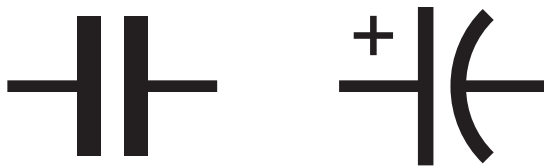
Figure 2-69. The generic schematic for a capacitor is on the left. The version on the right indicates a polarized capacitor which requires its left plate to be “more positive” than its right plate. The plus sign is often omitted.
