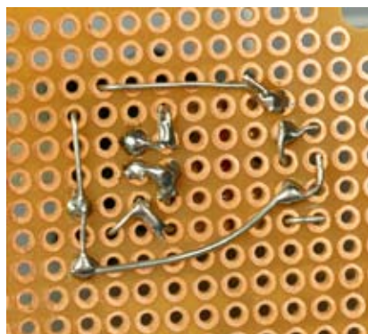
Figure 3-81. The assembly seen from below. The copper circles around the holes are not necessary for this project. Some of them have picked up some solder, but this is irrelevant as long as no unintentional short circuits are created.
