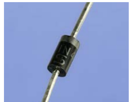
Figure 3-30. This 1N4001 diode is about 1/4 inch long and can handle up to 50 volts.
