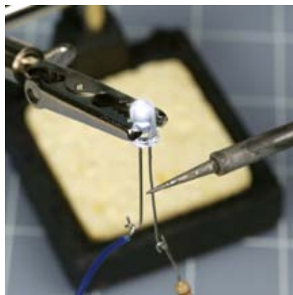
Figure 3-67. Applying heat with a 15-watt soldering iron. A typical LED should withstand this treatment for two or three minutes, but if you substitute a 30-watt soldering iron, the LED is likely to burn out in under 15 seconds.
