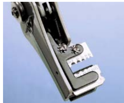
Figure 2-5. These automatic wire strippers enable one-handed operation, but are not suitable for very small wire diameters. See page 44.
