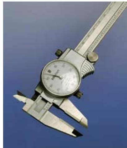
Figure 3-19. Calipers can be digital (which automatically convert from millimeters to 1/64 inch to 1/1,000 inch), or analog like these (so you never need to worry about a dead battery).
