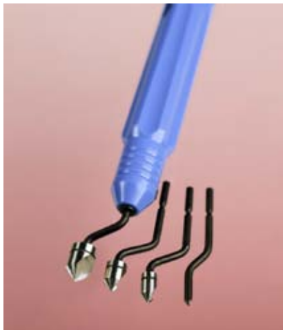
Figure 3-17. You spin this countersink tool like a hand crank to add just the right amount of bevel to a hole, so that it will accommodate a flat-head screw.
