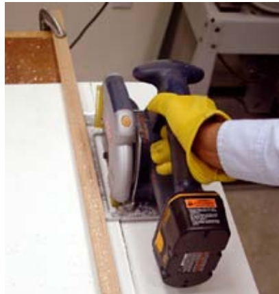
Figure 5-78. A handheld circular saw, running along a straight-edge, is much safer than a table saw for cutting plastic, and can produce comparable results.
