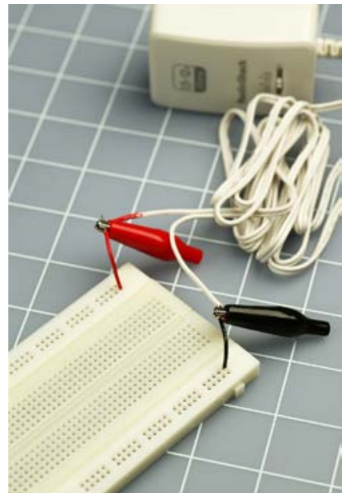
Figure 2-75. If your breadboard doesn't have screw terminals, insert two short pieces of solid-core wire with stripped ends and then attach the stranded wires from the adapter using alligator clips.
