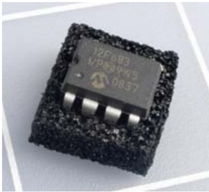
Figure 5-123. When supplied by one of its American distributors, a PICAXE 08M arrives embedded in a little square of conductive foam. The chip is the same size as a 555 timer but has the power of a tiny computer.
