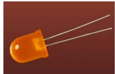
Figure 1-15. Jumbo-sized LED (1 cm diameter) is not necessarily brighter or more expensive. For most of the experiments in this book, buy whatever LEDs you like the look of.
