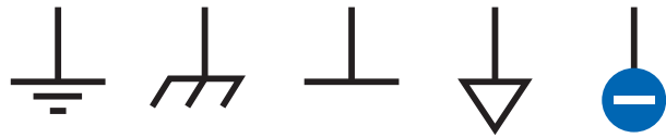
Figure 2-40. All of these symbols are used to mean the same thing: connect the wire to "ground" or "chassis" or the negative side of the power source. The far-right symbol is used in this book.
