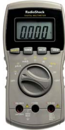
Figure 1-6. Mid-priced RadioShack meter, which has the basic features; however, the dual purpose for each dial position, selected with the SELECT button, may be confusing. This is an autoranging meter.
