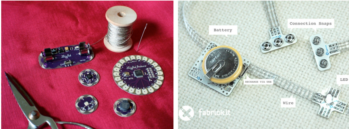
Figure 2. Kits that support making electronic textiles. Left: Lilypad toolkit (photograph by Leah Buechley). Right: fabrick.it (image by Despina Papadopoulou and Sascha Mombartz, fabrickit 2010 ©).
