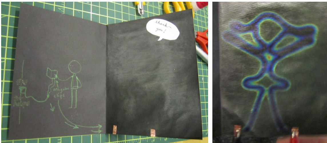
Figure 73. Thank-you note that reveals secret image in the liquid crystal ink when powered.
