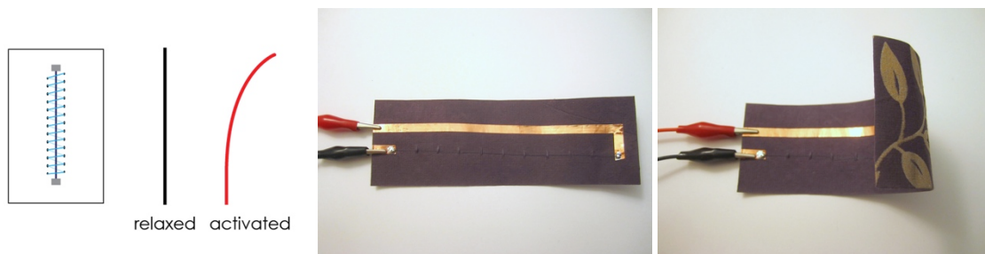
Figure 31. Curling mechanism diagram (left) with example in off (center) and on (right) states.
