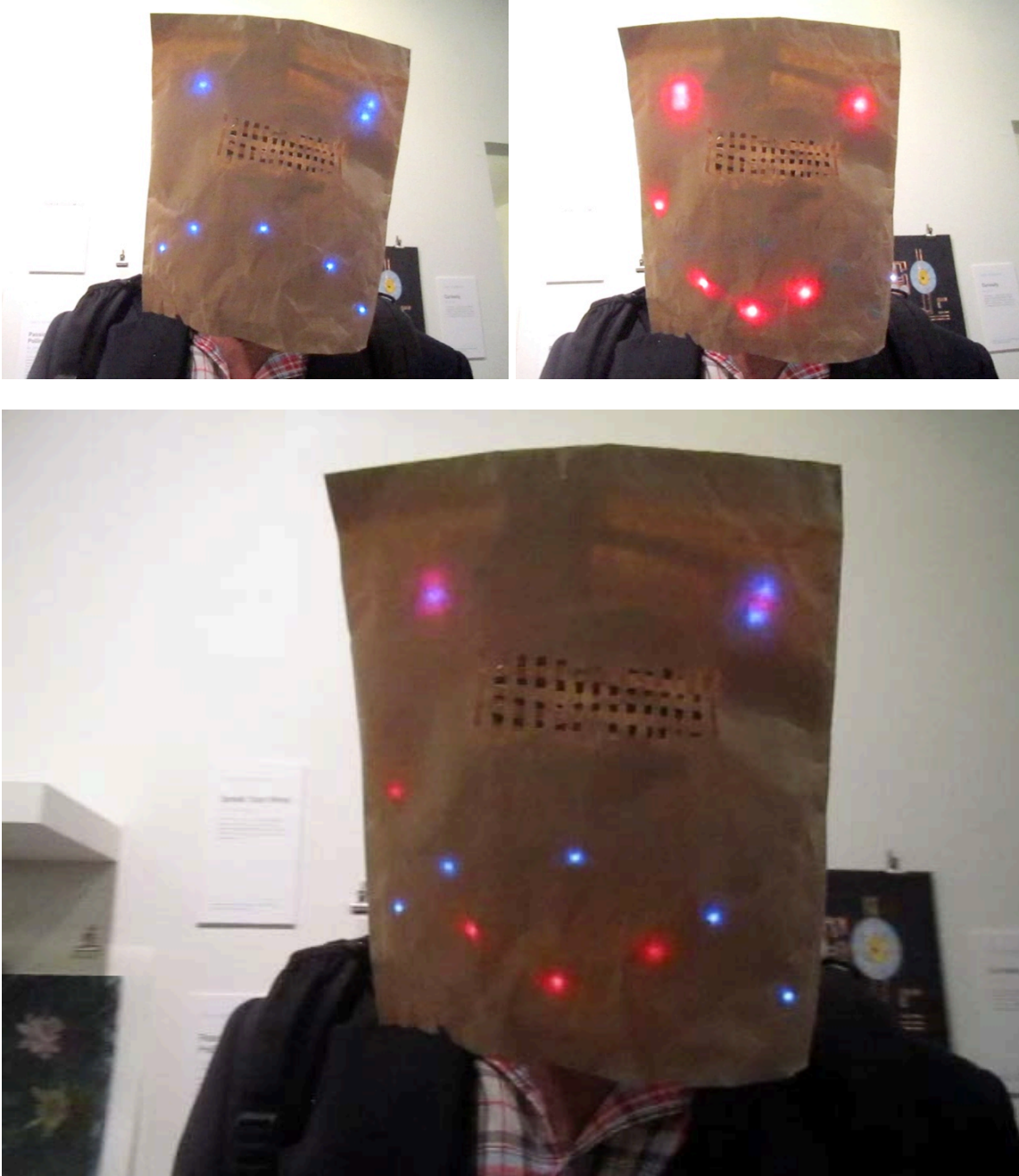
Figure 76. Speak Your Mind : a mask that changes expressions depending on the wearer's voice. The mask frowns when the wearer is quiet (above left) and smiles when the wearer yells into the mask (above right). Sometimes, the mask flickered quickly between the two expressions and appeared to have both (bottom), which happened often when wearers laughed into the mask.
