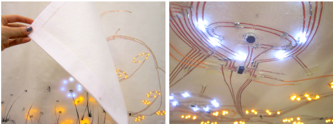
Figure 50. Attached with magnets, the painting can be peeled back (left) revealing the circuitry beneath it (right).
