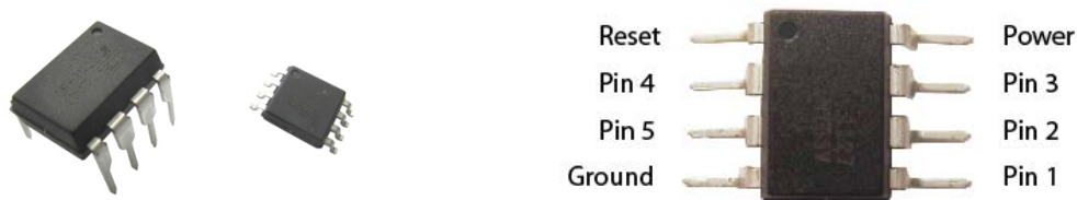
Figure 12. Attiny85 microcontroller in DIP and surface mount packages (left). Microcontroller pin numbering (right).
