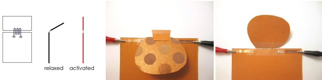
Figure 32. Straighten hinge mechanism diagram (left) with sample in off (center) and on (right) states.
