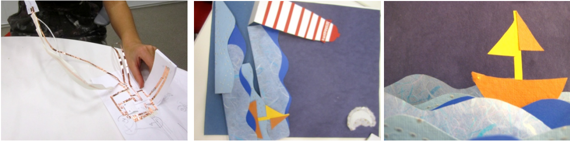
Figure 98. Lighthouse scene made by constructing the circuit (left) and crafting the scene (center) separately, and then integrating the two parts by sticking portions of the circuit onto the scene (right).
