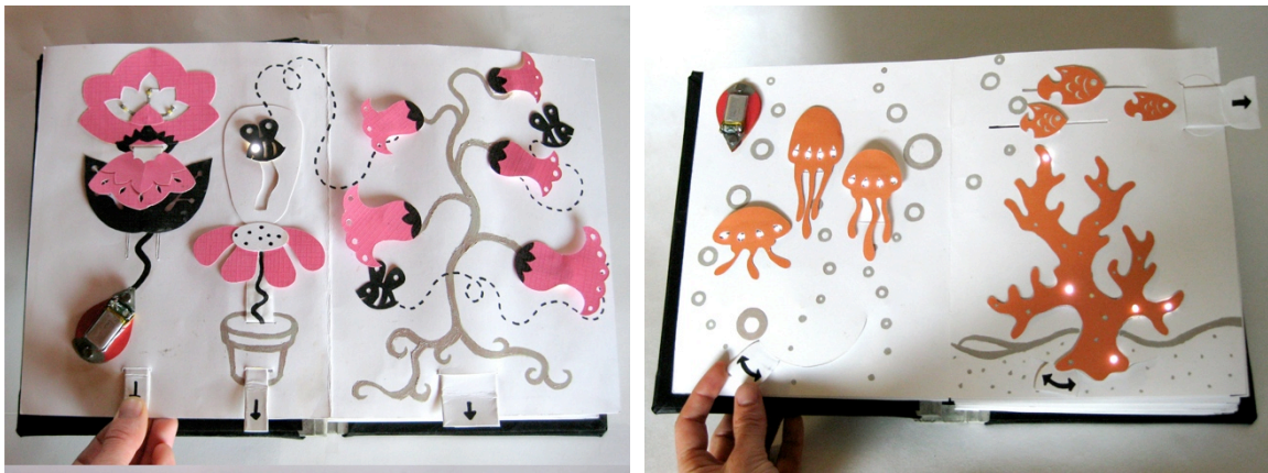
Figure 37. Flower-themed pull-tabs page (left) and underwater-themed potentiometers page (right). Photographs by Leah Buechley
