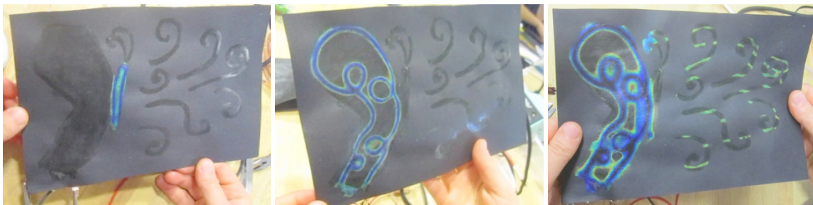
Figure 92. Discovering that the shortest thread heats up fastest (left). Using this technique to make the butterfly (center) appear before the gusts of wind (right).
