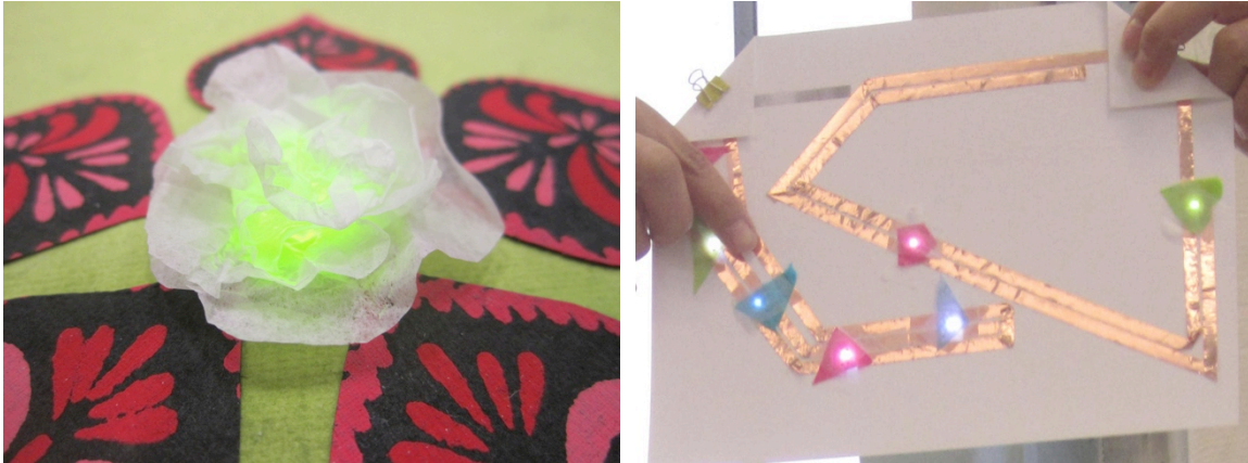
Figure 82. Tissue paper diffuser (left) and using colored papers to filter LED lights (right).
