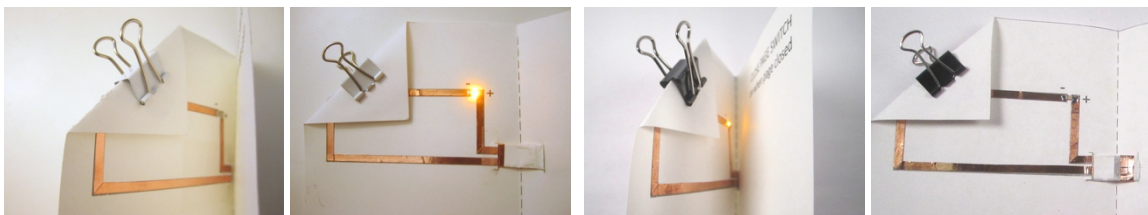
Figure 24. Attaching the slide switch across a fold allows it to detect page opening and closing. Depending on where the conductive band is placed on the slider, the switch can be turned on when the page is open (left) or when it is closed (right).
