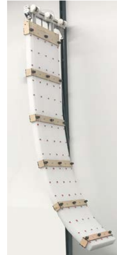
Fig. 1. Space Agent —a space-making (continuum) robot surface.
