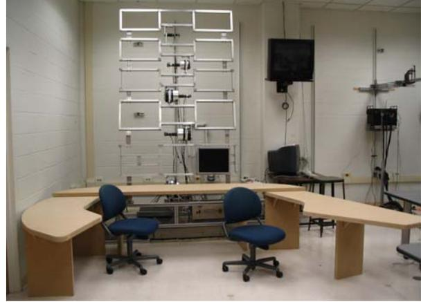
**Figure 2. The new AWE prototype.** [LEFT] *Eight aluminum frames and eight motors create the programmable “spine” of AWE. Larger computer displays occupy the lowest two frames; interchangeable panelized “tools” are “plug-and-played” into the upper six frames.*
