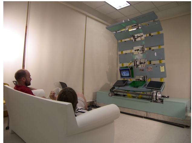
Fig. 9 AWE in lounging/viewing mode (configuration 6)
