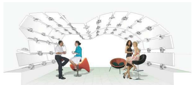
Figure 4: Animated Work Environment [AWE]. Rendering showing an application of the AWE system comprised of 2 sets of 4 co-joined AWE systems operating together at the scale of a large room (Authors).
