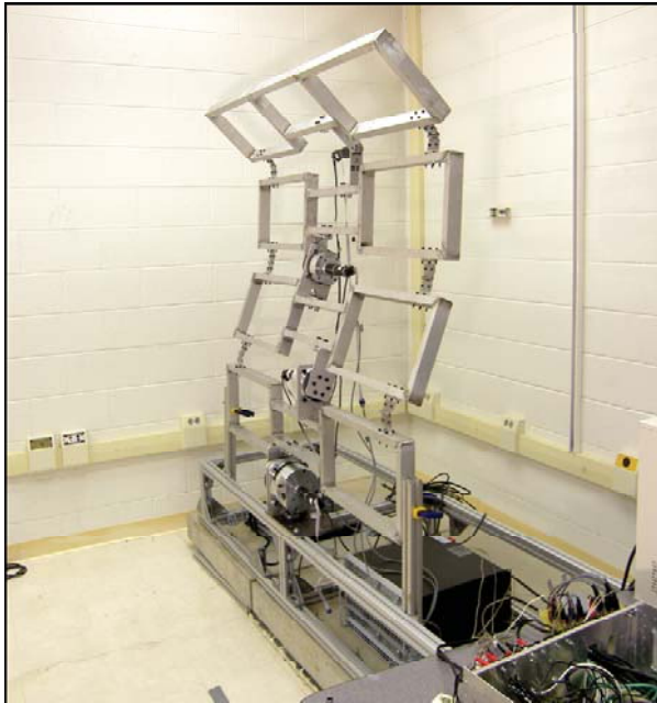
Figure 3: AWE. Developing prototype of the "Robotic Wall" Showing four of its eight panels (Authors).
