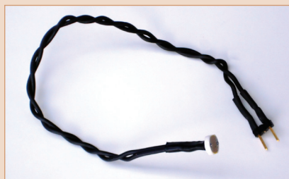
FIGURE A. Use male header pins to prepare connectors for easy interchange with your various projects. The connectors plug into a solderless breadboard.
